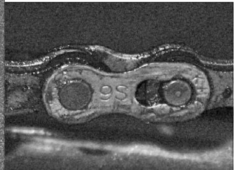
A master link disassembled (left) and assembled (right). A master link allows you to remove the chain without 'breaking' it.
