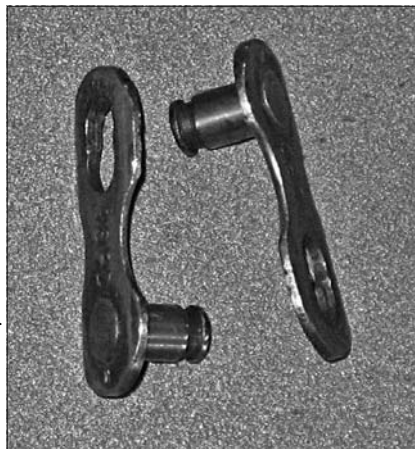
A master link disassembled (left) and assembled (right). A master link allows you to remove the chain without 'breaking' it.
